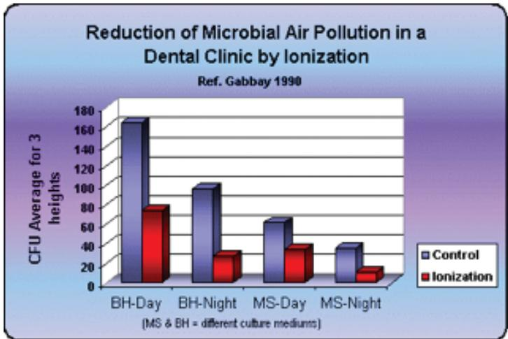
**Figure 1.** Reduction of microbial air pollution in a dental clinic by ionization (Pennsylvania State University, Aerobiological Engineering)
